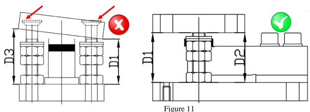
11. IF THERE IS A DEVIATION BETWEEN D1, D2 AND D3, THEN WE SHOULD PLACE METAL SHIMS OF DIFFERENT WIDTH (1,2 or 3mm) BETWEEN THE LEG OF THE SILO/TANK AND THE UPPER PLATE TO GET THE NECESSARY PARALLELISM FOR A CORRECT INSTALLATION (Figure 12)
